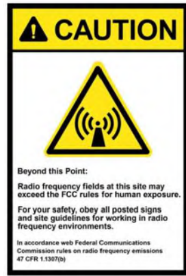
1 CAUTION SIGN - 12" X 8" -PLACED ON TOWER -USE A DECAL ON MONOPOLE AND METAL SIGN ON SELF-SUPPORT TOWER OR GUYED TOWER
