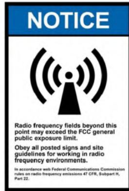
3 RF GUIDELINES SIGN - 12" X 8" - PLACED ON FENCE
