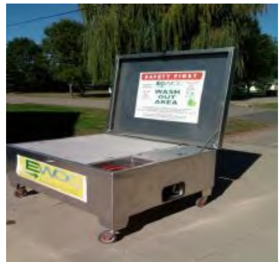
Self-Contained Washout Facility
