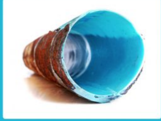
old pipe repaired with new lining
